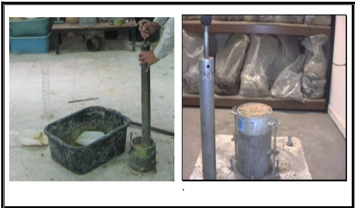
Figure 5.7 Proctor compaction test devices
