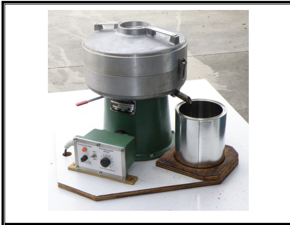
Figure 5.10 Centrifugal Extraction machine
