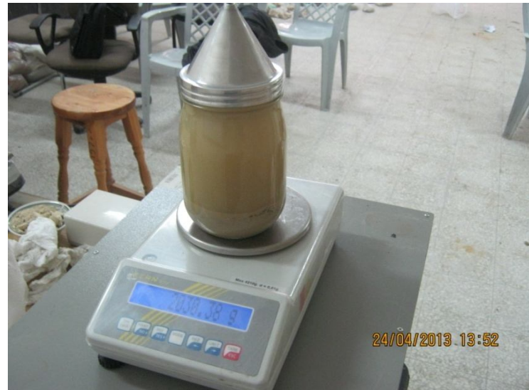
Figure ( 4 ) : Determining specific gravity for fine aggregates by Pycnometer.
