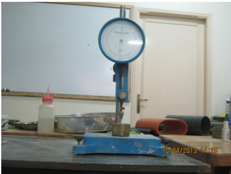
Figure ( 7 ) : Penetrometer device for Liquid limit test.
