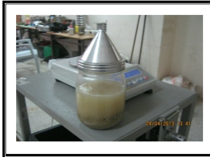
Figure 5.2 Pycnometer device for determining specific gravity
