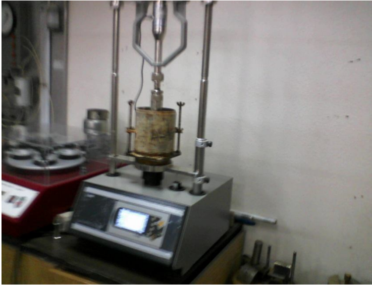
Figure ( 5 ) : CBR test device
