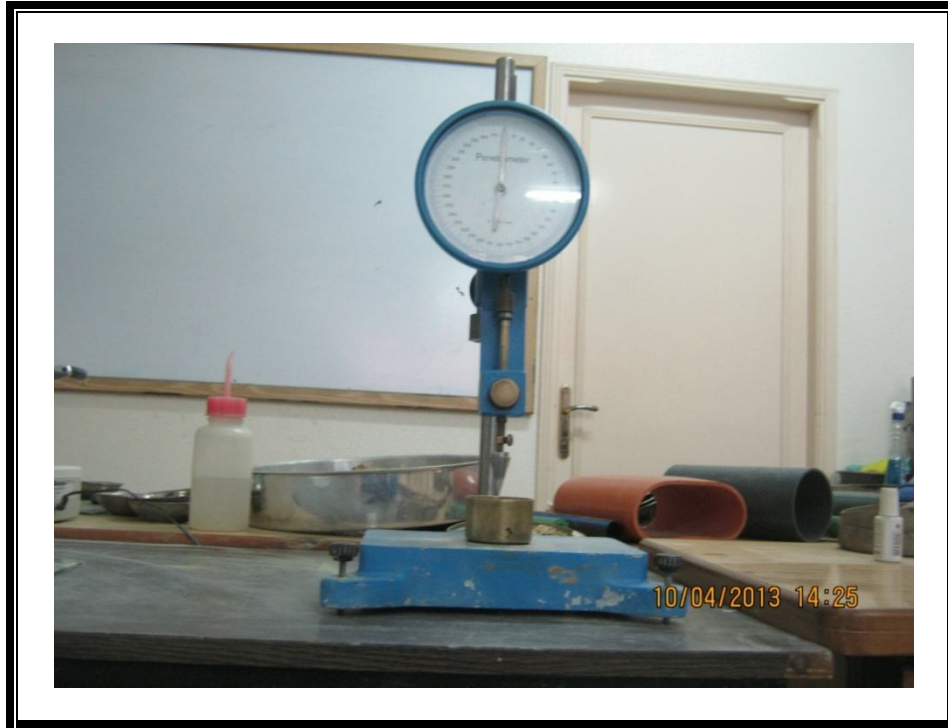
Figure 5.3 Penetrometer device for determining liquid limit
