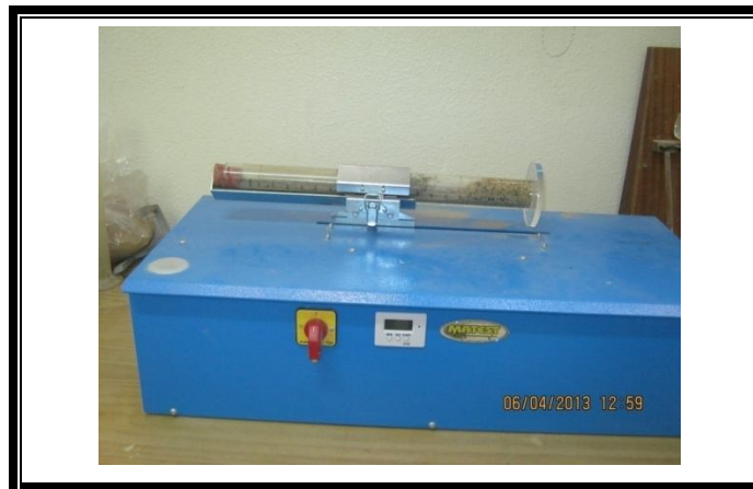
Figure 5.5 Mechanical shaker device for sand equivalent test
