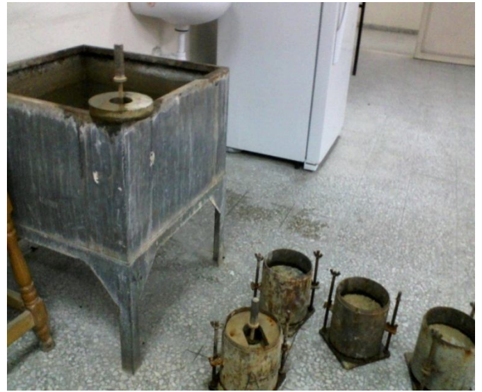
Figure ( 6 ) : CBR molds
