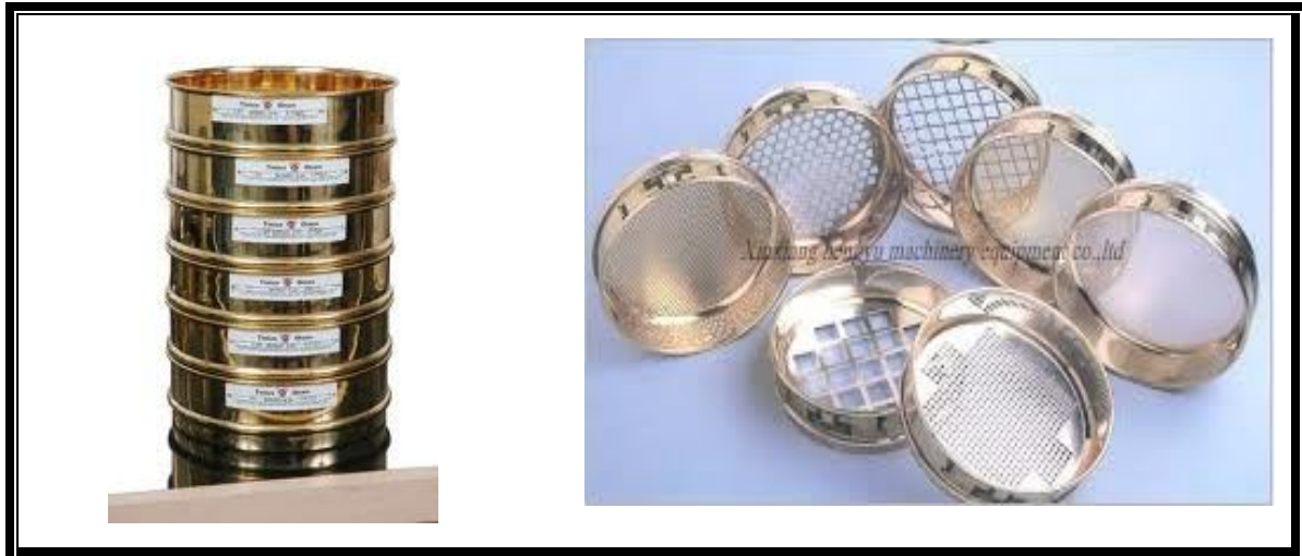
Figure 5.1 Gradation test standard sieves devices
