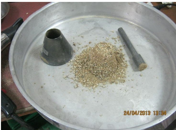
Figure ( 3 ) : Cone tools for determining saturated surface dry condition.
